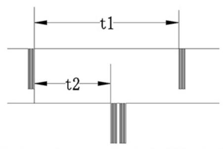
Remark: Control command code is 0X01, t1≥250ms t2=200~210ms When the command code is 0X10~0X13, t1≥100ms t2=65 ~75ms
