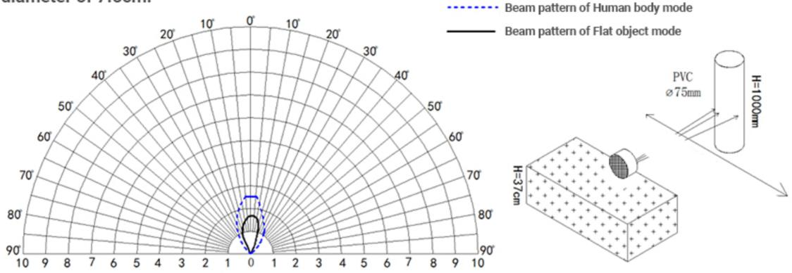
(2) The tested object is a corrugated box perpendicular to the 0° central axis, with a length \* width of 60cm\*50cm.
