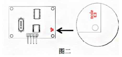
The module has two measurement modes: plane and human body which set by hardware. The module can be set to different measurement modes by changing the circuit board mode and setting the resistance value.
