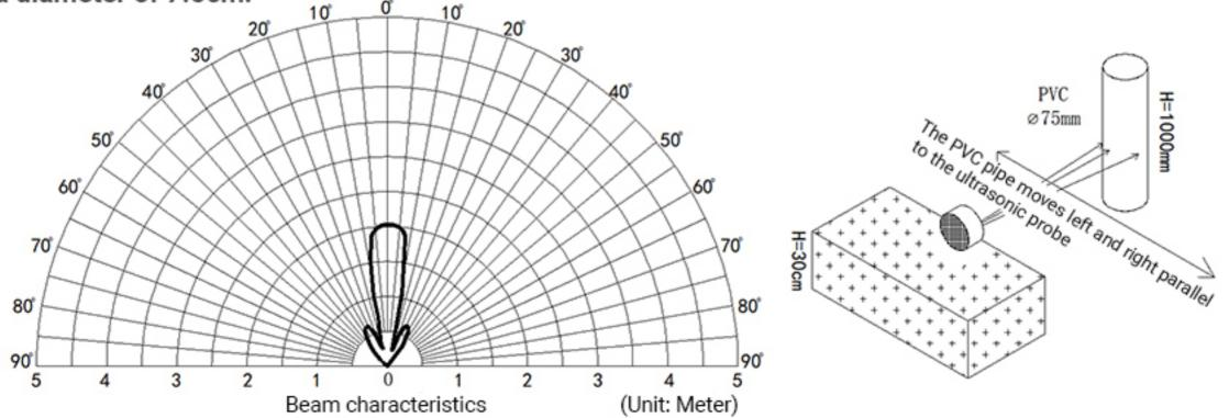
(2) The tested object is a corrugated box perpendicular to the 0° central axis, with a length \* width of 60cm\*50cm.
