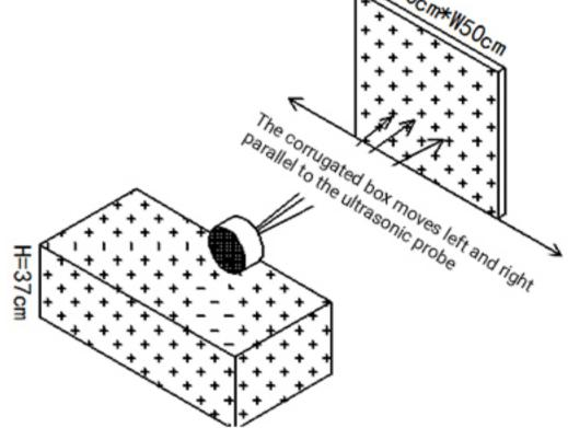
(3) The tested object is a corrugated box tangent to the arc, length \* width is 60cm\*50cm.
