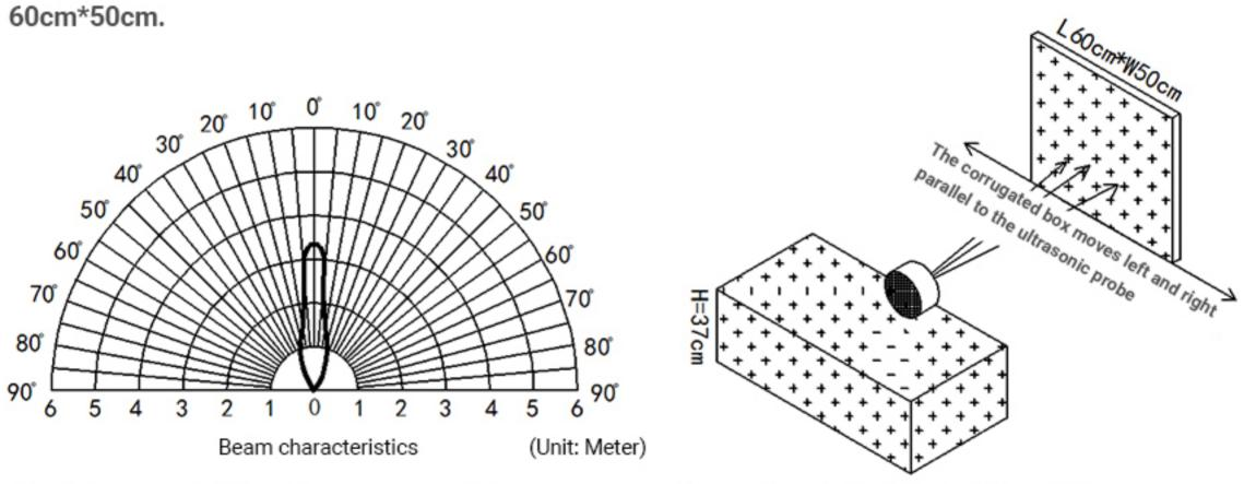
(2) The tested object is a corrugated box tangent to the arc, length \* width is 60cm\*50cm.
