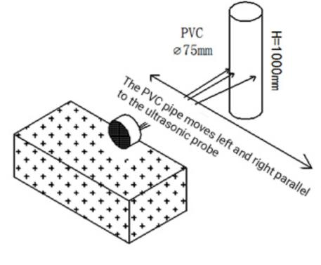
(2) The tested object is a corrugated box perpendicular to the 0° central axis, with a length \* width of 60cm\*50cm.
