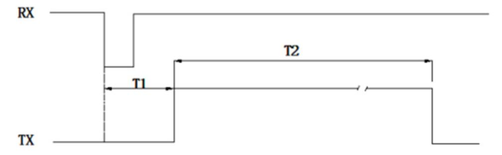
Remark: T1=12~16ms; T2=1.4~32ms(Duration of high level PWM)
