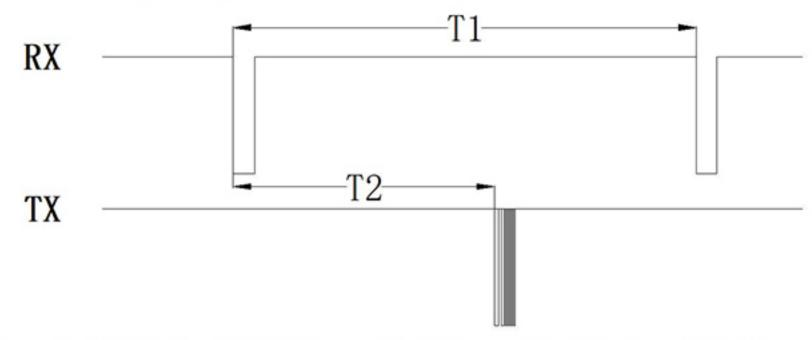
Remark: A13 Series T1>500ms, T2≈380ms; A13B Series: T1>60ms, T2≈31ms
