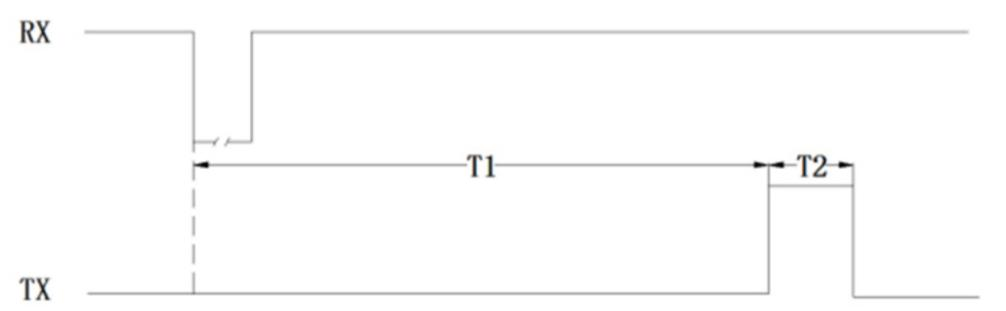
Remark: A13Series: T1≈380ms, T2=1.4~25ms. A13BSeries: T1≈30ms, T2=1.4~25ms
