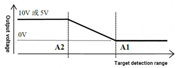
Remark: The resistive load of the analog voltage output is ≤10mA.
