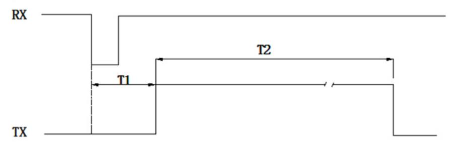
Remark: T1≈100ms T2=1~35ms (Timing of PWM High-level pulse width)
