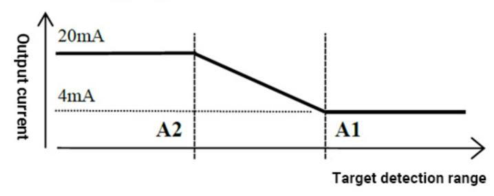
Remark: The resistive load of the analog current output is ≤300Ω.
