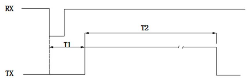
Remark: T1=10~17ms, Flat object mode: T2=0.18~35ms(Timing of PWM High-level pulse width)
