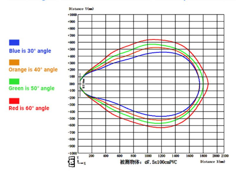
2Vertical angle: The central connection of the two probes is arranged vertically to the ground.
