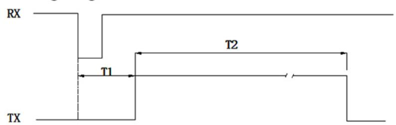
Note: T1=5 $\sim$ 8ms (measured in non dormant mode); T2=0.18 $\sim$ 30ms(PWM high-level pulse width time); a pulse width of 10us was detected for the output of the same frequency interference.
