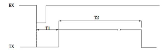
Note: T1=5 $\sim$ 8ms (measured in non dormant mode); T2=0.18 $\sim$ 30ms(PWM high-level pulse width time); a pulse width of 10us was detected for the output of the co-frequency interference.
