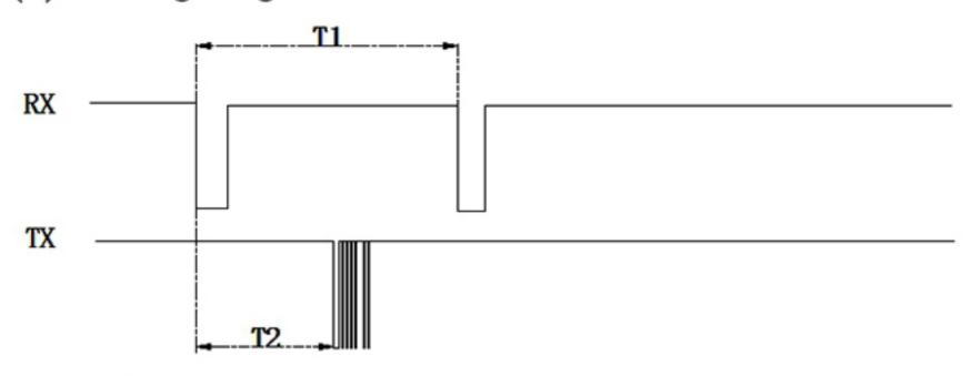
Note: T1 > T2+15ms; T2=8 $\sim$ 140ms; measured in non dormant mode.
