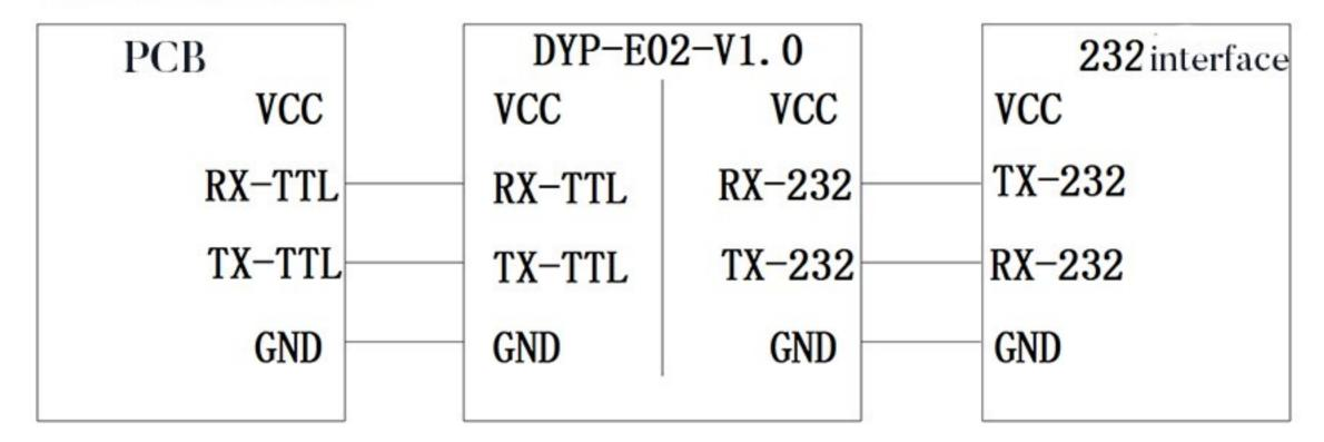
Remarks: The VCC pin can be connected or not connected according to the actual application.
