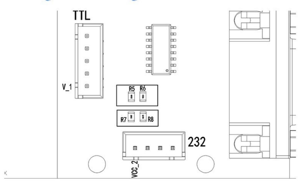
When R5 is welded with 0R resistor, R6 position is floating, VCC\_1 pin is connected to VCC\_0 pin, and the voltage of VCC\_1 pin is equal to the supply voltage of VCC\_0 pin. When R5 position is floating, R6 position is welded with 0R resistor, VCC\_1 The pin is a 5V voltage output.
