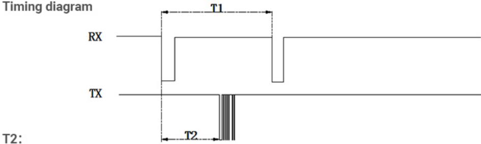
Mode 1:  $(28+2*(response time of interface ranging module+12))\sim(28+2*timeout);$
