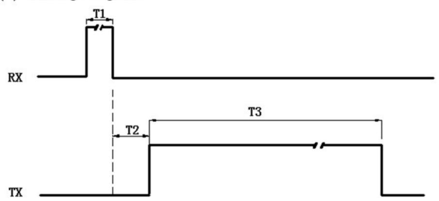
Remark: T1=0.1~10ms; T2=4.5~6.0ms; T3=0.55~65ms (Timing of PWM High-level pulse width)
