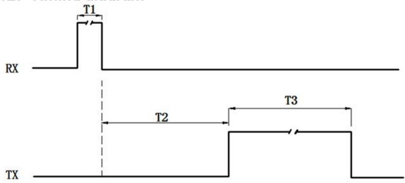
Remark: T1=0.1~5ms, T2≥75ms, T3=0.6~65ms (Timing of PWM High-level pulse width)
