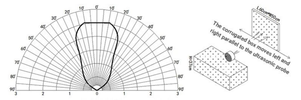
(3) The tested object is a corrugated box tangent to the arc, length \* width is 60cm\*50cm, the solid line in the figure below is the module's default angle test data; the dotted line is the small angle mode test data.
