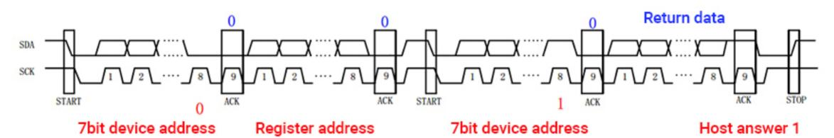
(2) Read 2 bytes of data, with the high eight bits first and the low eight bits behind
